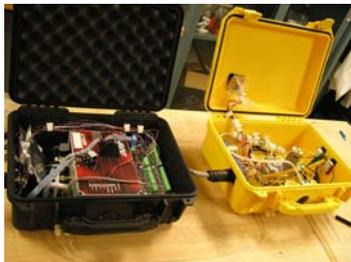
Fig. 1. Schematic diagram and photograph of ship-based  $\text{CO}_2$  /  $\text{O}_2$  monitoring system.
