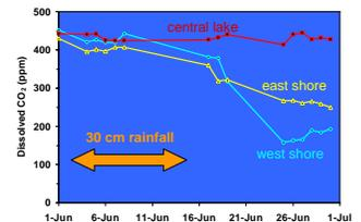
Fig. 4. Plot showing the temporal development of the spatial  $\text{CO}_2$  pattern shown in Fig. 3. Following the rain event, the  $\text{CO}_2$  concentration remains relatively constant at mid-lake, but decreased dramatically near the shores.
