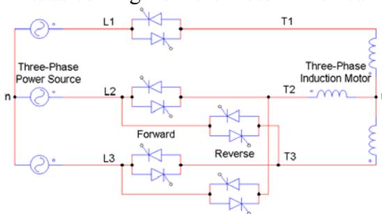
**Figure 17: Reversing Soft Starter Topology**
