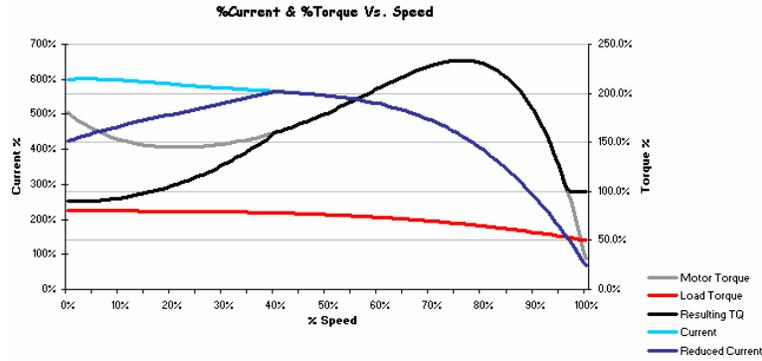
Figure 22: Soft Start Motor Starting Characteristics [8]
