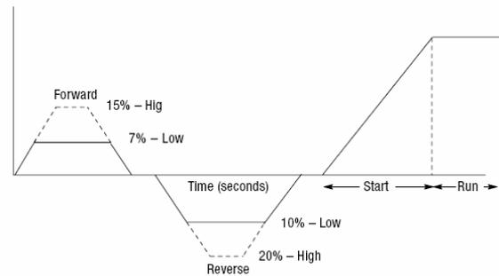
Figure 34: Low Speed and Low Speed Reversing Profile [7]
