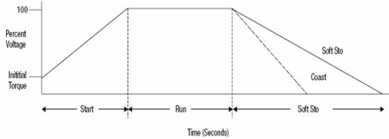
**Figure 14: Voltage Ramp [7]**
