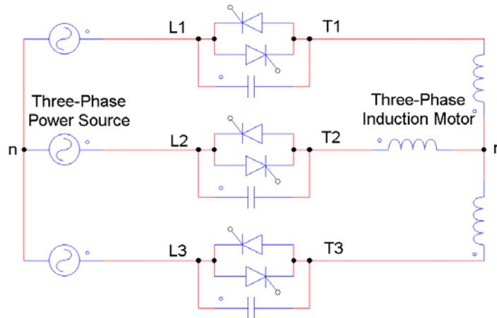
**Figure 5: Standard Soft Starter Topology With Bypass**
