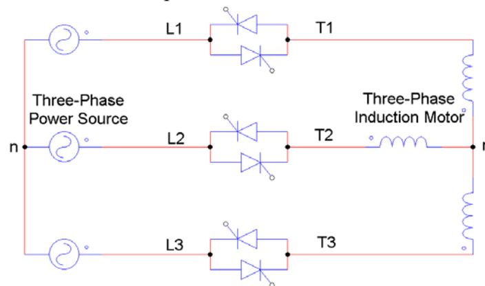
**Figure 1: Standard Soft Starter Topology**
