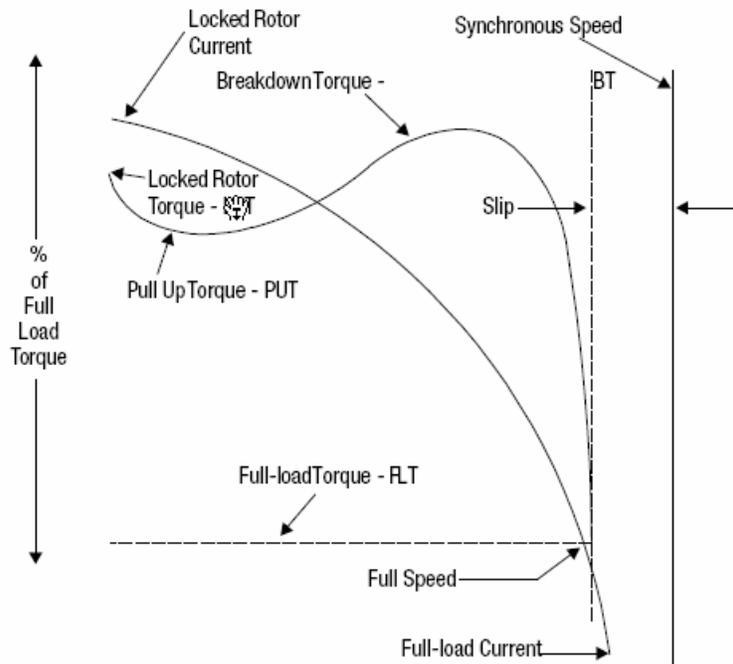
Figure 35: Speed/Current vs. Torque Curve Explanation [7]
