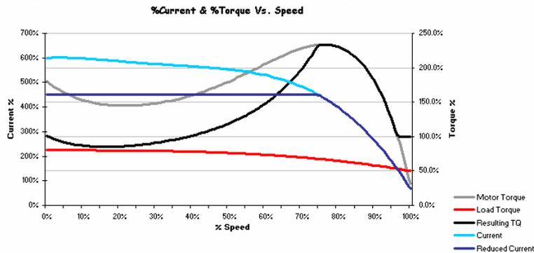
Figure 23: Current Limit Motor Starting Characteristics [8]
