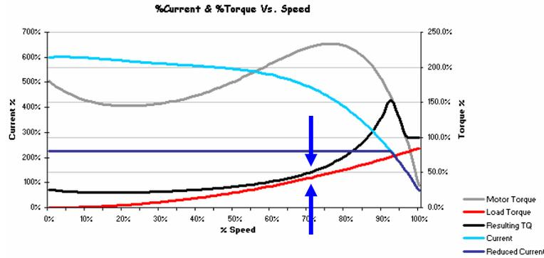
Figure 29: Pump Current Limit [8]
