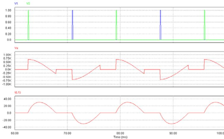
**Figure 9: Single Phase Simulation (90° Firing Angles, Voltage, and Current)**
