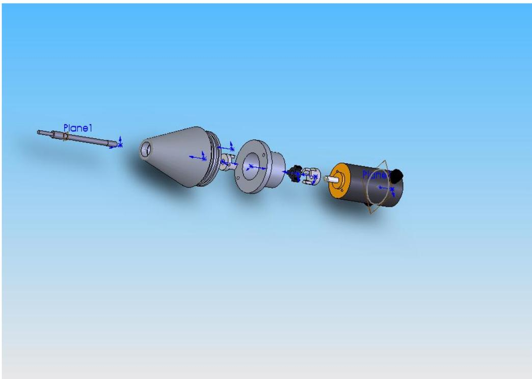
**Figure 8: Shaft Assembly Exploded View**
