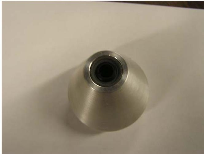
**Figure 2: Shaft Seal**
