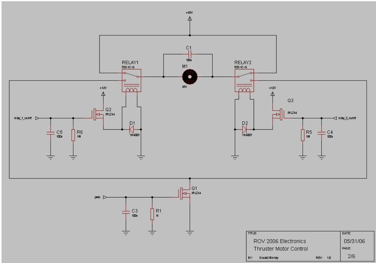
Figure 14: Thruster Circuit
