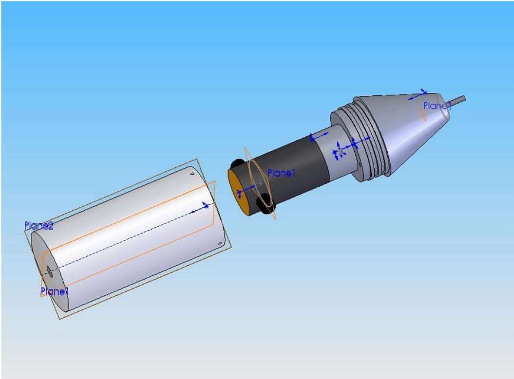
**Figure 7: Thruster Exploded View**
