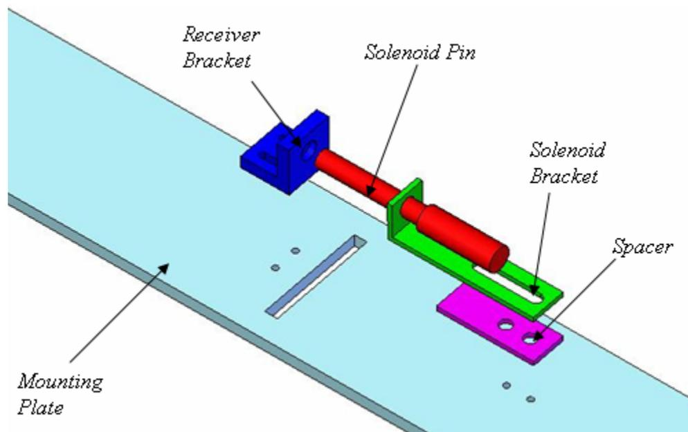
**Figure 9: Electronics Module Delivery System**
