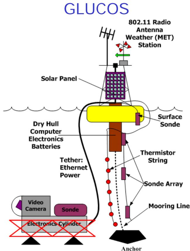
Figure 20: GLUCOS Buoy Layout
