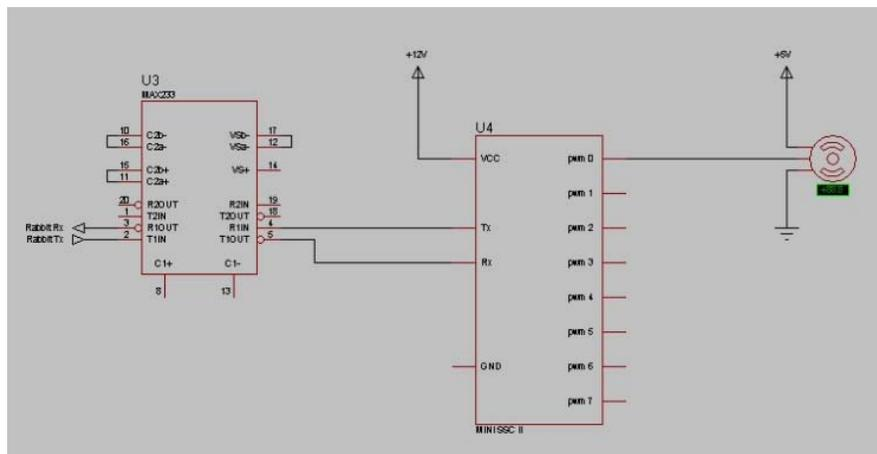
Figure 13: Servo Controller
