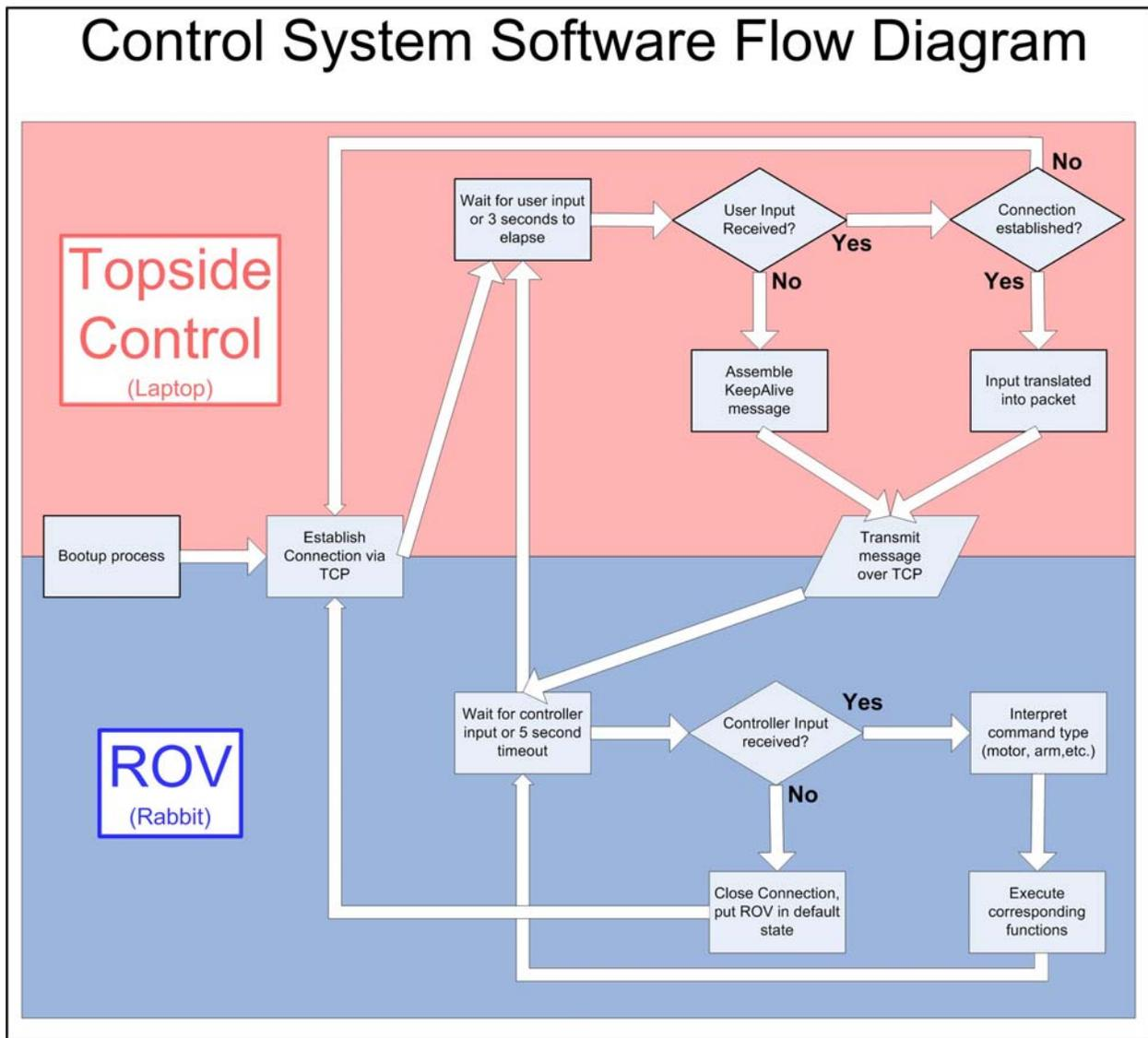
**Figure 18: Software Flow Diagram**
