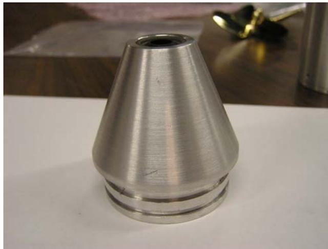
**Figure 6: Thruster Cone**
