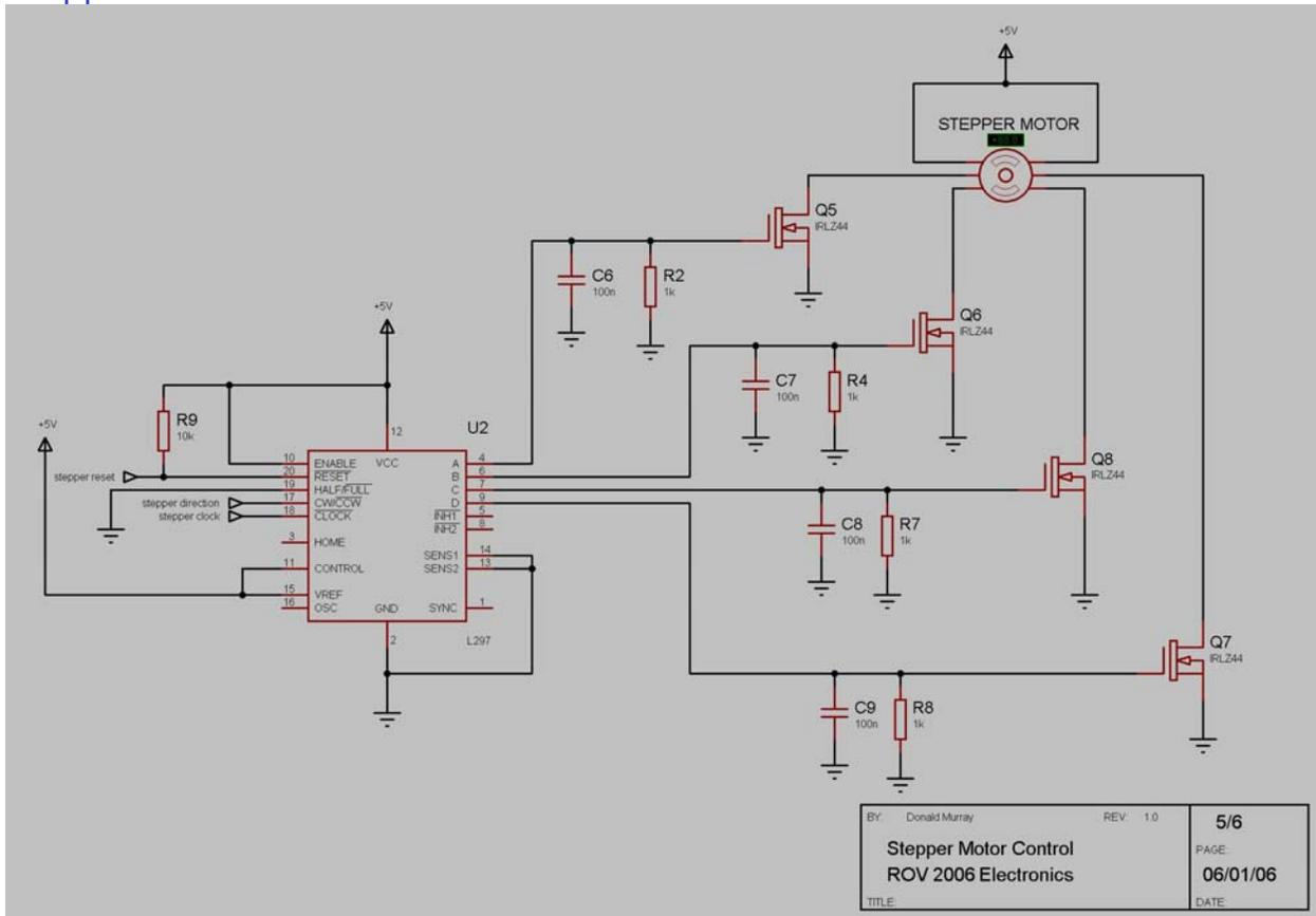
Figure 15: Stepper Motor Circuit
