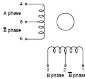
Figure 2: Typical Unipolar/Bipolar Stepping Motor Wiring
