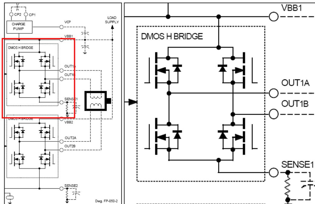
**Figure 10: H-Bridge configuration Internal to A3977SED**
