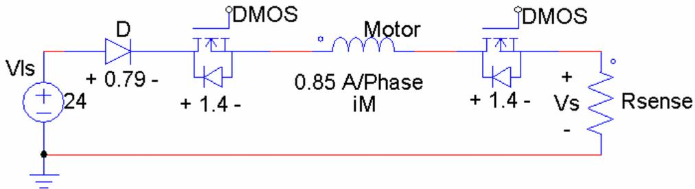
**Figure 9: Motor Circuit Path One Phase**
