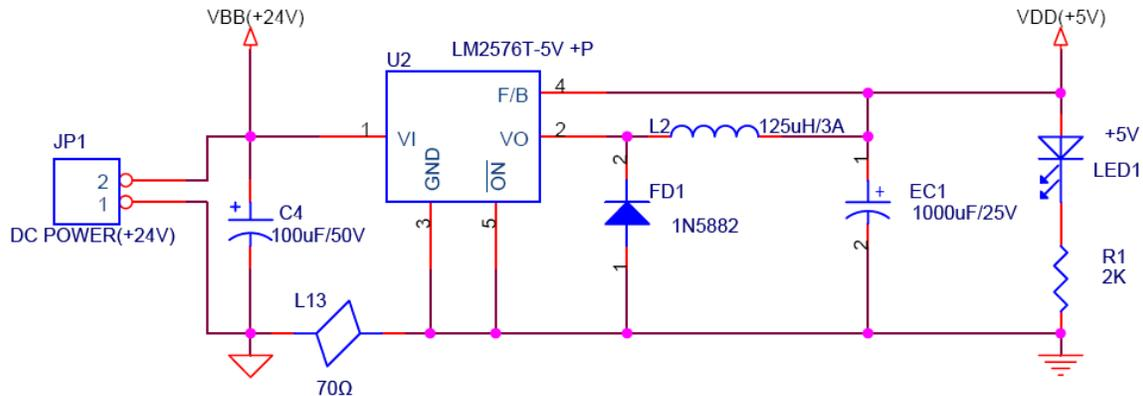
Figure 3: Implementation of LM2576-5V
