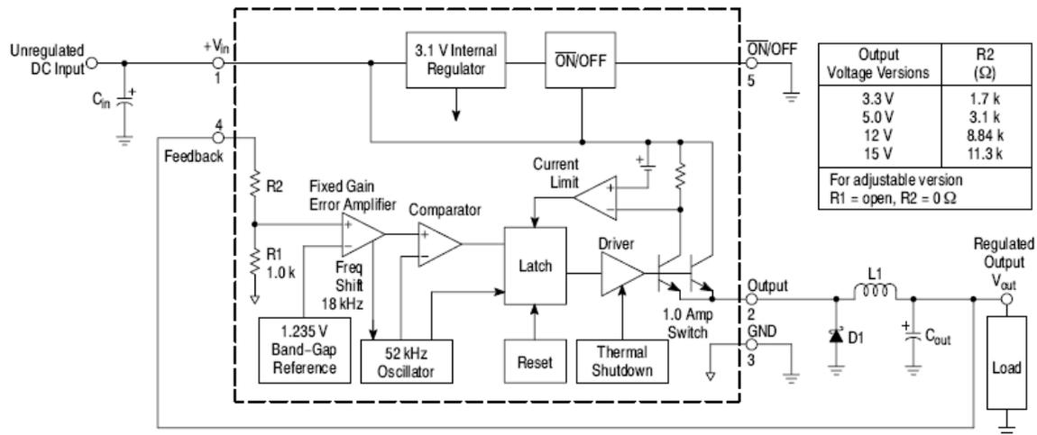
**Figure 4: Internal Block Diagram of LM2576-5V**
