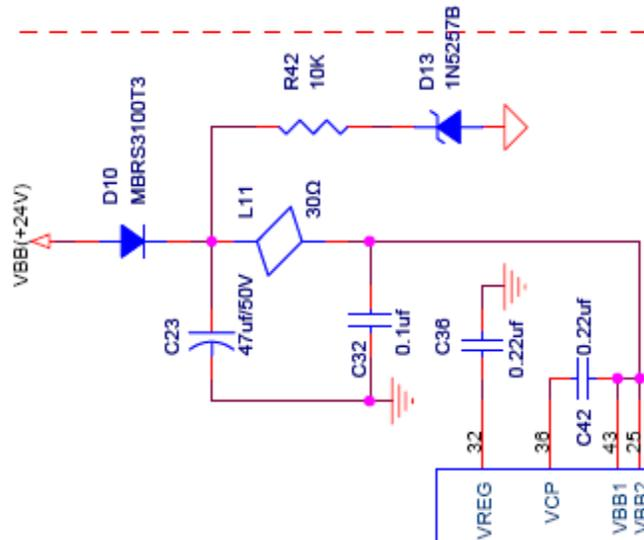
**Figure 12: Regulation Circuit for Motor Supply Voltage**
