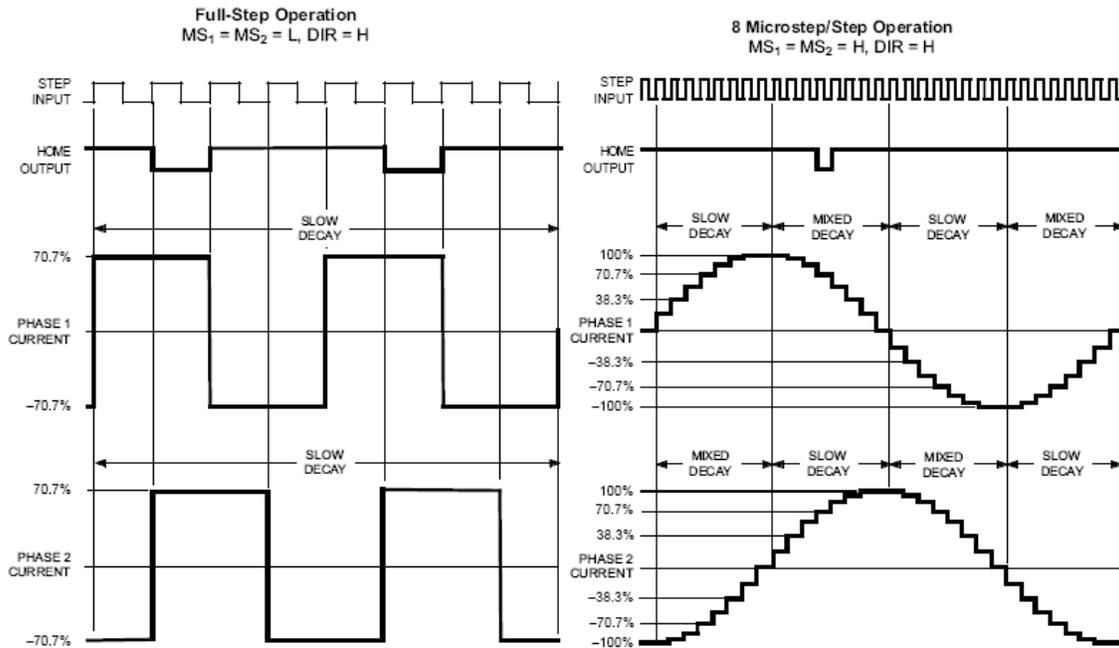
Figure 15: PWM Switching Currents for 1 Step Rotations and 8 Step Rotations
