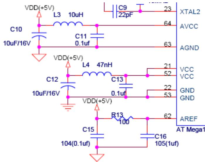
**Figure 14: Input Voltage Filters**
